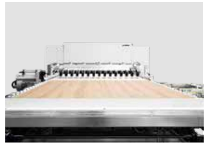
Rip cut panel dividing
